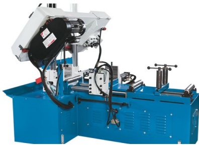
Bundle vise is provided for cutting entire material material to length
