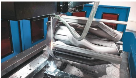
In additive production (3D-Printing) the produced complex parts are attached to a metal plate, where the metal plate subsequently will have to be separated from the component (Neospark 500 B Continental Engineering Services)
