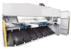
*With the optional pneumatically controlled plate hold-up fixture even thin metal sheets can be positioned with high accuracy at the back gauge*
