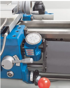
The thread gauge allows for resuming the thread after the apron nut for retrograde motion has been opened
