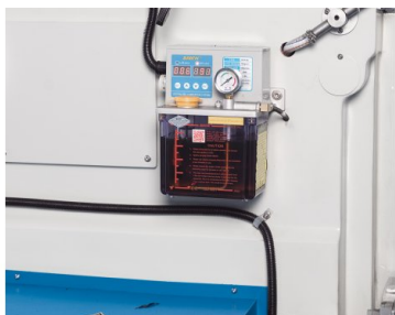
Automatic central lubrication reduces maintenance
