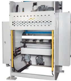
A large throat and narrow table ensure plenty of free space to accommodate complex bending
