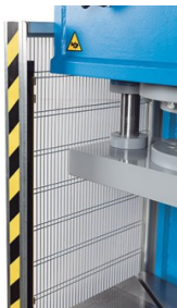
The workspace is protected by light curtains
