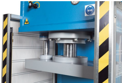
The workspace is protected by light curtains
