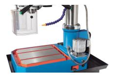
The coolant pump is integrated in the machine base
