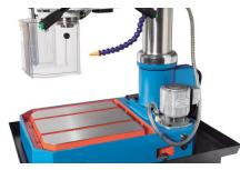
The coolant pump is integrated in the machine base
