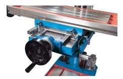
A rigid compound sliding table ensures precise positioning of hole patterns and drill patterns
