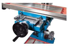
A rigid compound sliding table ensures precise positioning of hole patterns and drill patterns
