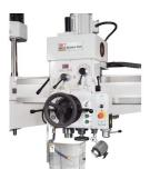
Speed is infinitely variable across 2 levels and shown on the display
