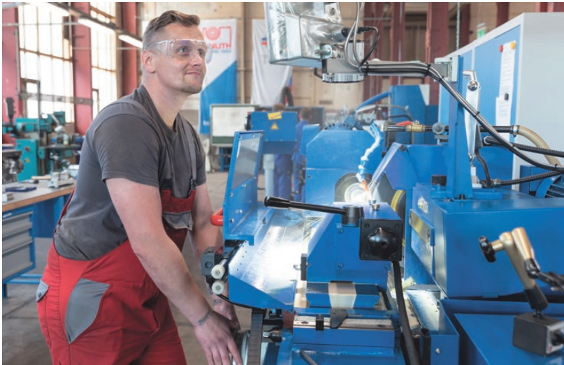
Trainees learn how to produce top-quality surfaces and dimensional stability through cylindrical grinding.
