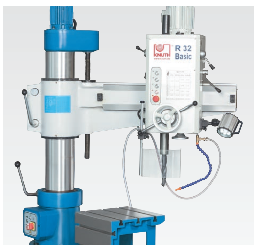
Swiveling boom for large throat widths
