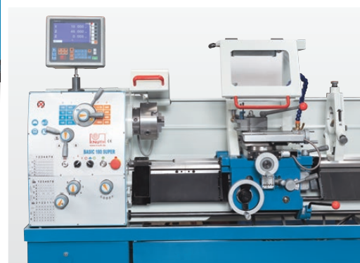
Select the optimum spindle speed for the Basic 180 Super via its 16-step main drive
