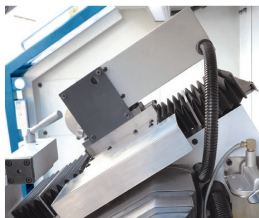
Inclined bed design optimizes work space and chip removal
